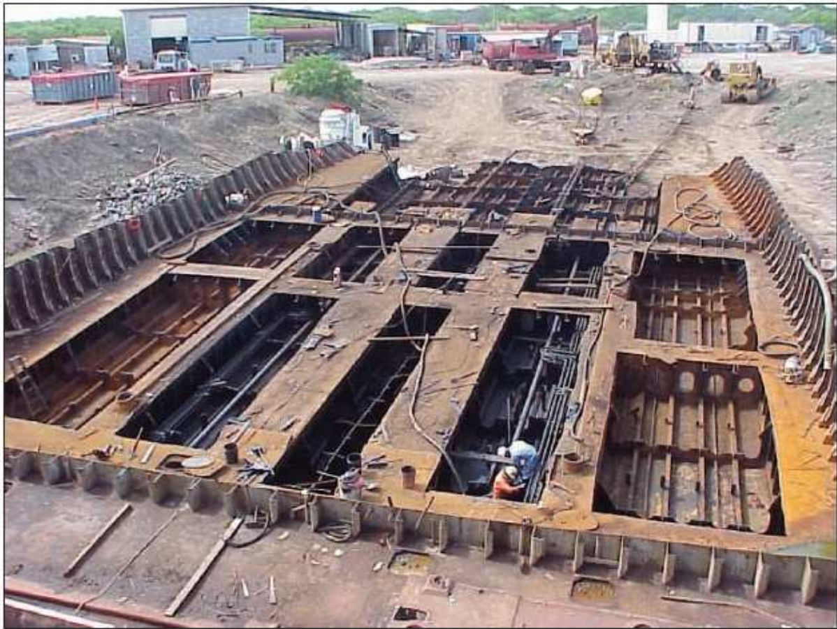
Figure 3: Ship Near End of the Scrapping Process
