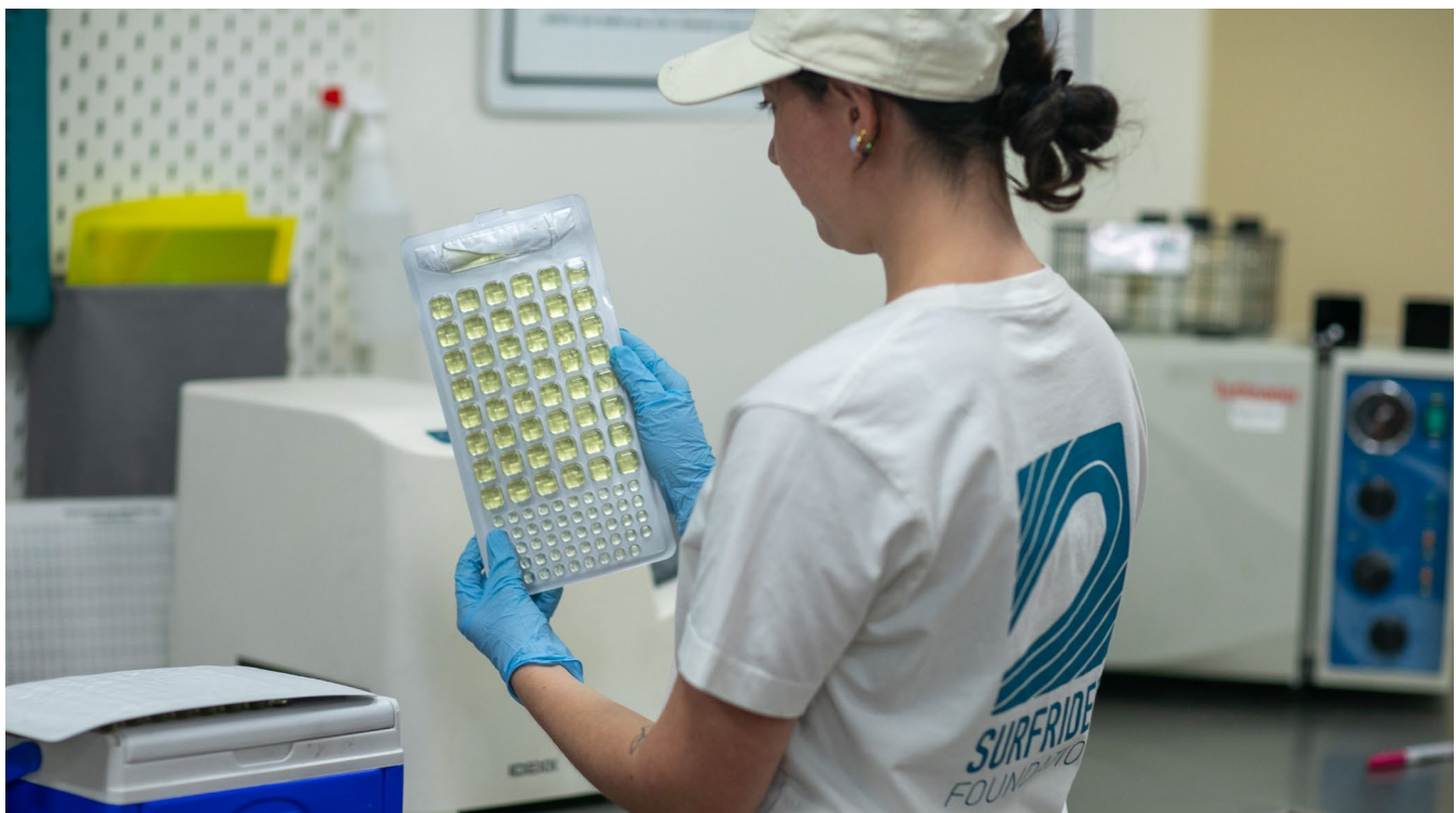
Water quality samples are sealed in a multi-well tray before being placed in the incubator.
